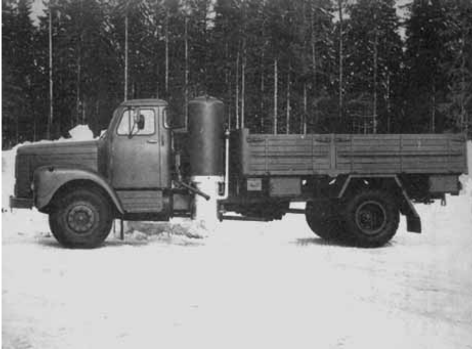
Figure 3.13 Picture of a Scania L8050 truck converted to wood gas operation
